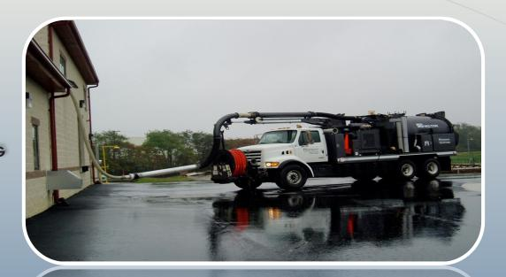
Our 8-foot telescoping boom lets the operator position the 8" suction tubes up to a 90-degree angle for far reaches from the truck, while the water pump delivers up to 80 gpm @ 2,500 psi for jetting operations. The 600' hose reel telescopes and rotates for optimum positioning for jet rodding sewers.
